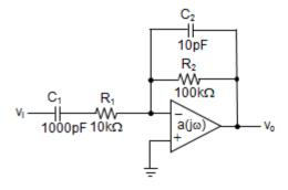
A feedback amplifier is made using an operational amplifier as shown above. The open-loop transfer function of the operational amplifier  $a(j\omega)$  has a DC gain of 100dB and two poles at 100Hz and 10MHz.
