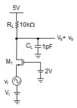
In the CMOS amplifier shown above, answer with the following parameters:  $\mu C_{ox} = 200 \mu A/V^2$ ,  $V_{th} = 0.4 V$ , and W/L = 200.
